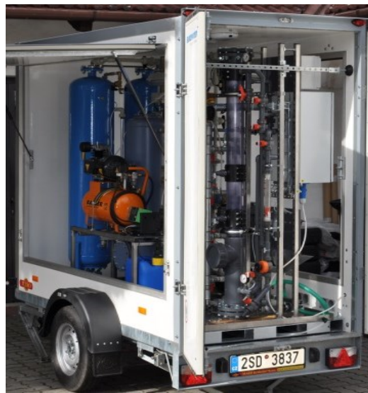
Figure 1: Mobile Pilot Water Treatment Plant
